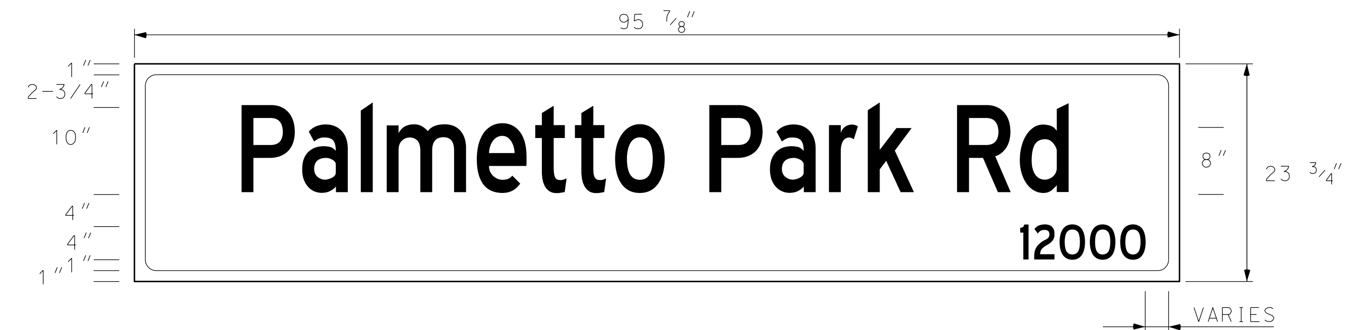
ILLUMINATED STREET NAME SIGN TYPICAL (LONG NAME) DIVIDED STREET NAME OR T-INTERSECTION ADD BLOCK NUMBER ON THE SAME SIDE AS INTERSECTING STREET
